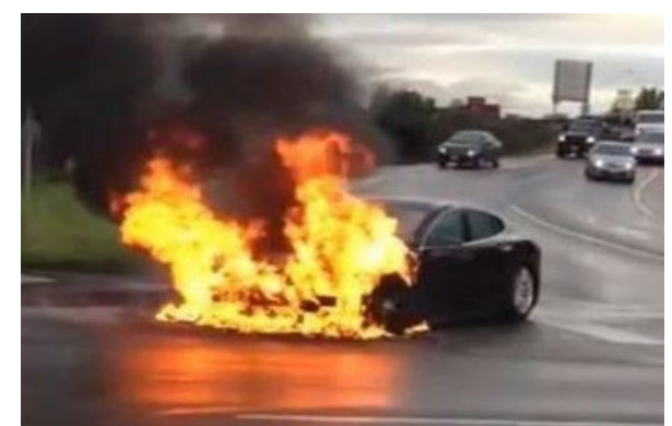
Vehicle fire caused by heat chain of a battery
